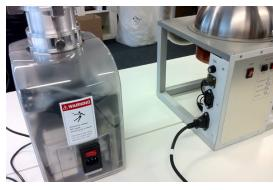
26. Connect brown power cable between vacuum pump and measuring stand
