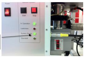
38. After finish of working to stop system: Push "Stop" button for few second...
