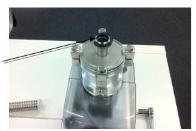
7. Mount vacuum valve with use of vacuum clamp
