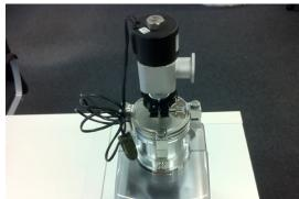
8. Connect vacuum pipe with use of vacuum clamp
