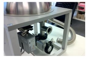
11. Connect other side of vacuum pump to flange onto measuring stand
