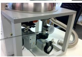
10. Remove cover from flange of vacuum pipeline
