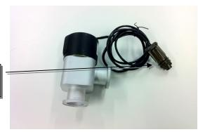
17. Take electronic block. Back side. Connect yellow alarm cable
