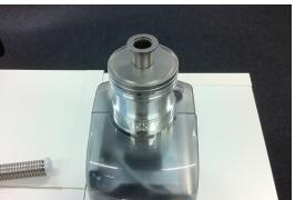
5. Mount interconnector with use of four vacuum fixtures
