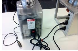
27. Connect cable with special connector of vacuum gauge to measuring stand.
