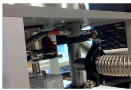
30. Look from bottom of measuring stand. Connect blue sygnal cable as shown
